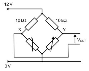
The variable resistor is set to a resistance of  $12 \,\mathrm{k}\Omega$ .
