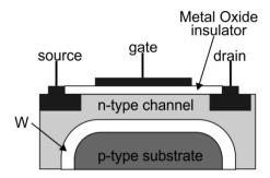
The n-type channel is separated from the p-type substrate by a region, labelled W, which contains virtually no free charge carriers.
