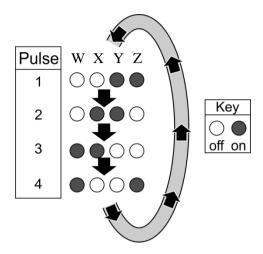
The LEDs are controlled by a counter and logic system, controlled by pulses from an astable sub-system as the block diagram shows.
