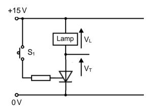
(i) Complete the table by adding the values of  $V_L$  and  $V_T$  when switch  $S_1$  is closed and immediately re-opened. The thyristor is initially switched off. [3]
