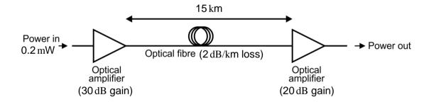
Calculate the power leaving this section of the communication system. [4]
