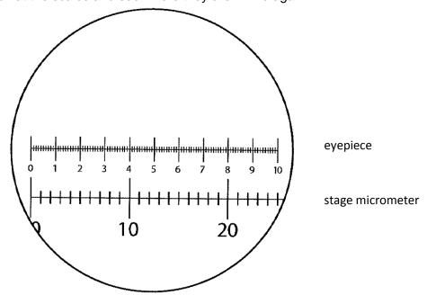
Using this x40 objective lens, 20 stage micrometer units make up 80 eyepiece units.
