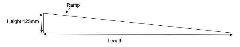
Note: The ratio of the height of the ramp to the length is 1:15
